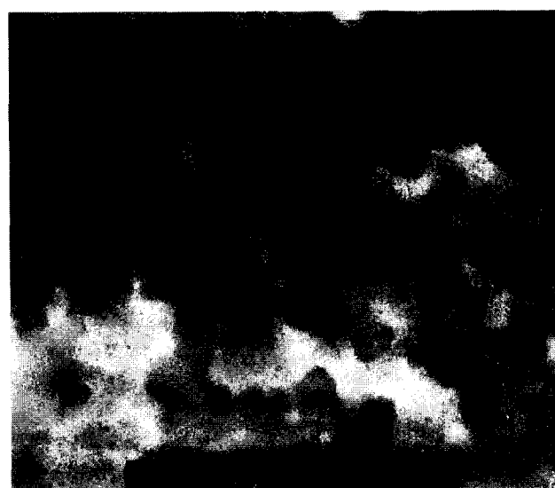
Figure 3 Transmission electron micrographs of polyurethane/allyl diglycol carbonate interpenetrating polymer network, PU content 30%: (a) TMP = 0.0 equivalents, magnification 50 000; (b) TMP = 0.4 equivalents, magnification 50 000; (c) TMP = 1.6 equivalents, magnification 30 000
